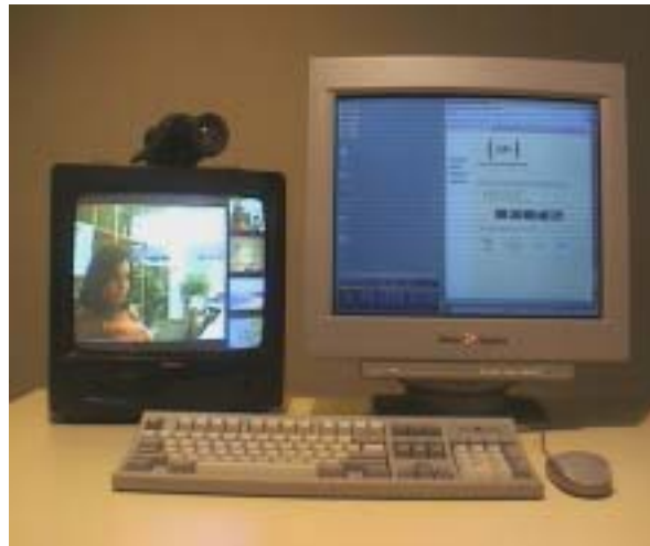
Figure 1. Typical configuration for an analog mediaspace node
